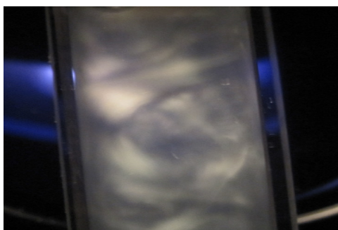
Figure 40. Shear-induced birefringence in the aqueous suspension of N-methylmorpholine betaine ester of CNC viewed through crossed polarizers, concentration ~0.05% w/w.
