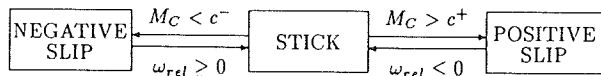
Figure 3.6: Phase switch conditions of a single clutch. “>” should be read “becomes greater than”.
