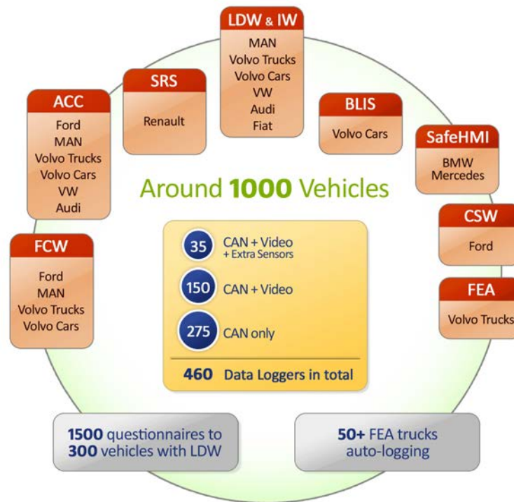
Figure 2: Overview of systems and data loggers in euroFOT
