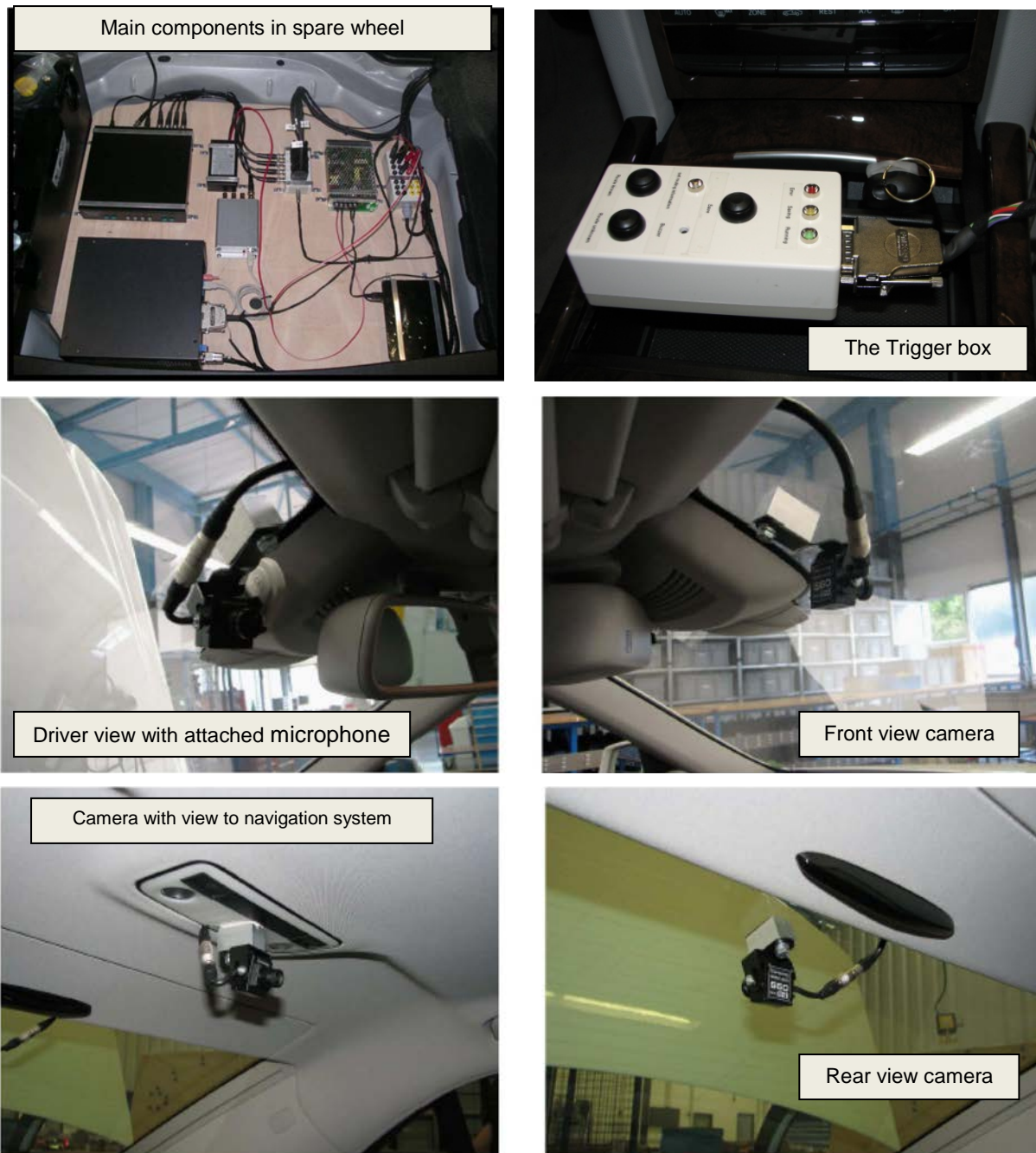
Figure 15: Placement of DAS in a Daimler vehicle.
