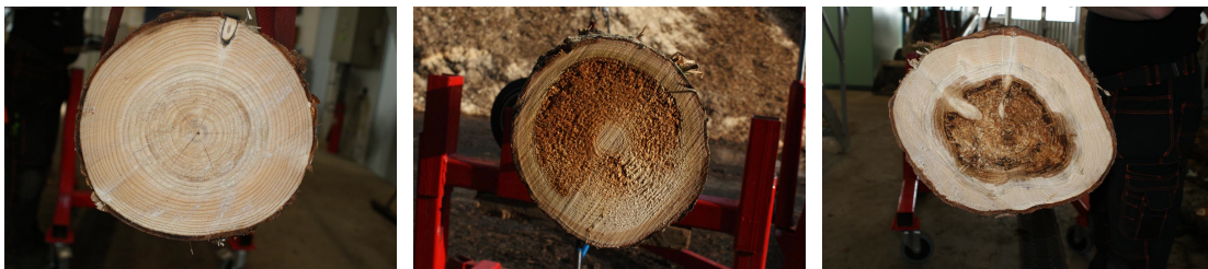
Figure 1.11: This picture shows an example of (a) perfectly healthy log, (b) half rotten log and (c) rotten log
