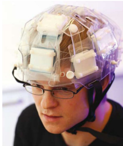
Figure 1.8: The measurement device used in the stroke type detection project.
