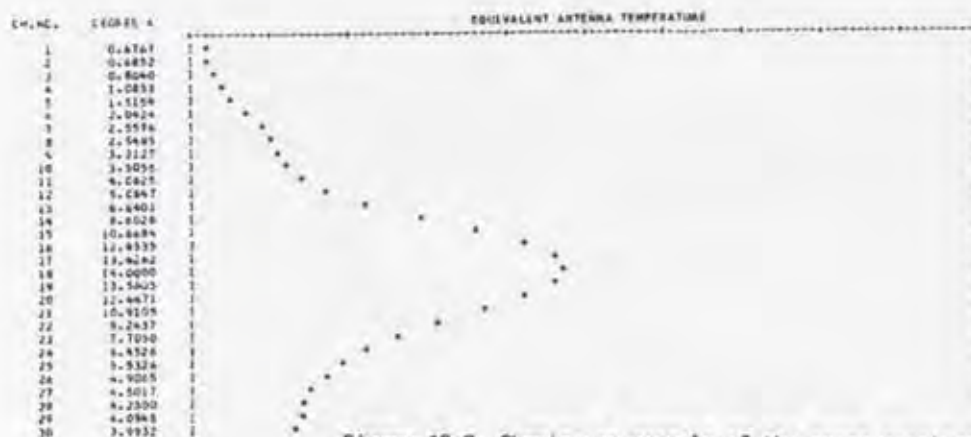
Figure 10.2 Showing an example of the power spectrum of an OH signal obtained by means of the AUTOCORR program. Total bandwidth 6 kHz. Spectrum 1. Zero line + W3 OH radiation Spectrum 2. Zero line + 3C273 radiation Spectrum 3. Normalized spectrum of the -43.7 km/s, right circular polarized W3 OH radiation.
