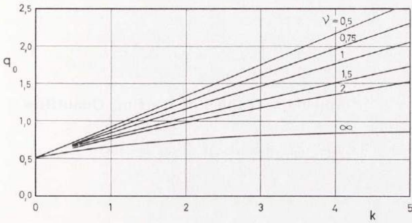
Chart 17.1. Oil Flow q_0 = \frac{q}{U h_{\min}}
