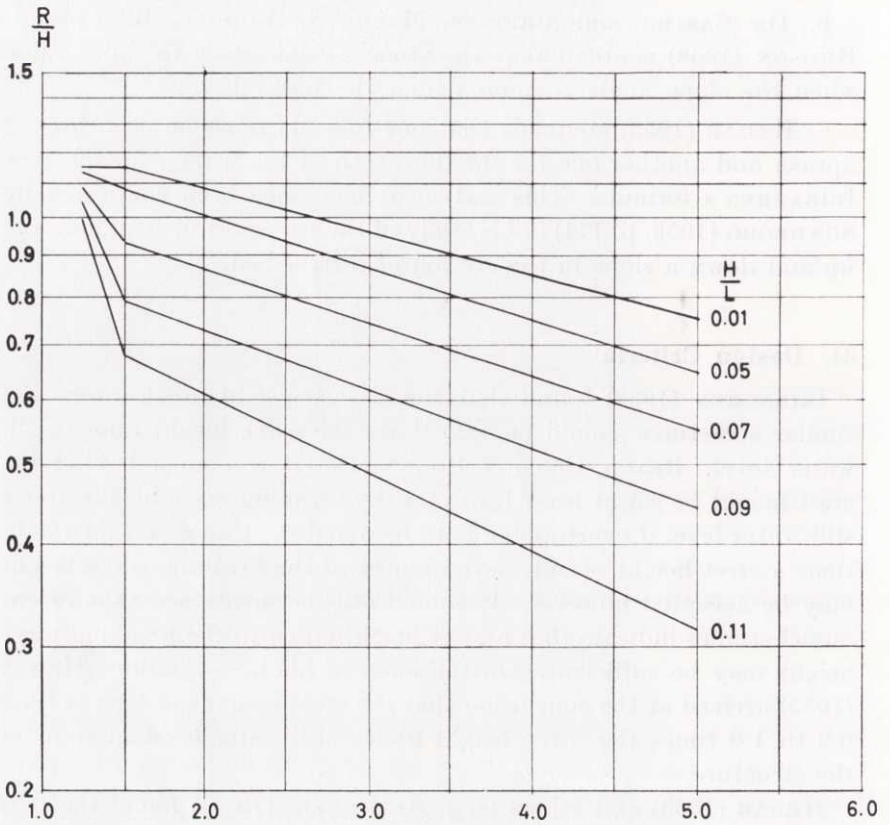
Fig. 34.1. The ratio of run-up to wave height, \frac{R}{H} , as a function of \cot \alpha with the wave steepness \frac{H}{L} as parameter. (After HUDSON (1958, 1959) )
