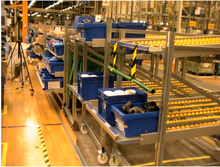
Figure 3.13. A photo showing one of the stationary cameras and the gravity flow racks used in the experiment in Study II
