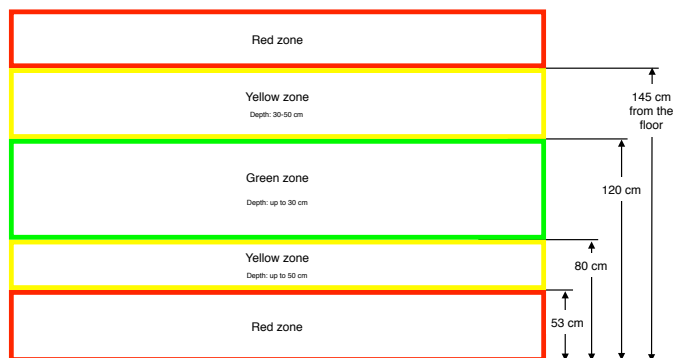
Figure 3.5. The schematic plan of the VASA model, coding exposure positions as green, yellow, and red (including the height from the floor and depth at the different levels)
