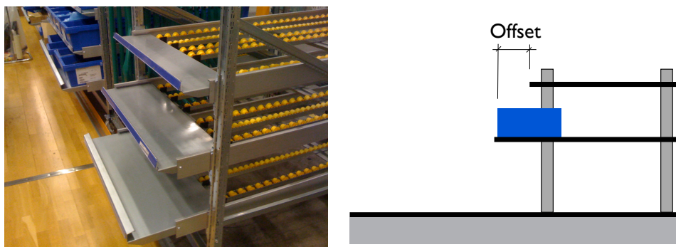
Figure 4.6. Vertical offset is depicted to the left and the schematic is to the right
