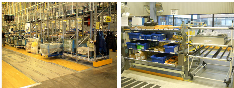
Figure 3.8. On the right is a photo of the redesigned materials exposure applied by the case company primarily based on plastic containers in gravity-flow racks, and on the left is the original materials exposure primarily based on wooden pallets with wooden frames in pallet racks.
