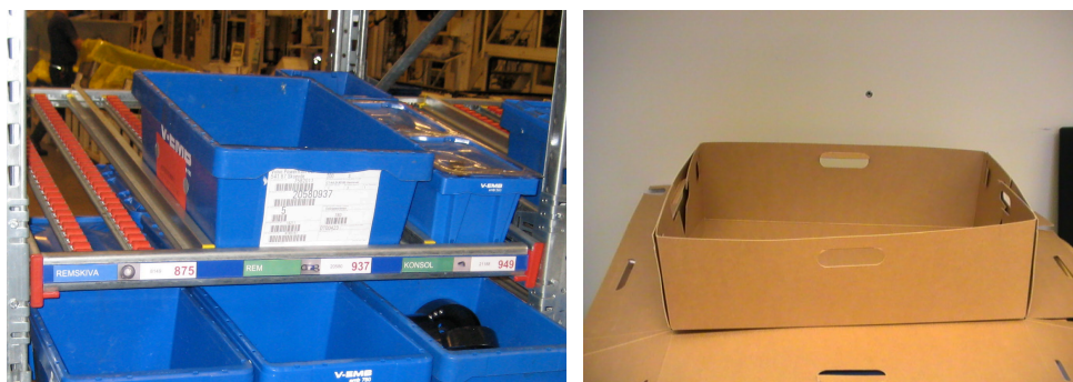
Figure 3.12. To the left: the re-usable plastic packaging used in the case. To the right: the developed one-way cardboard packaging.
