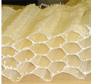
Figure 6. A three-dimensional hollow woven structure with uneven surface (Chen, 2009).
