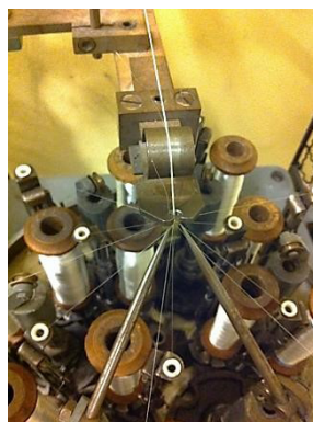
Figure 3. A circular braiding machine with twelve cones interlacing for braiding.
