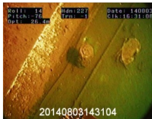
Tank cap of bronze at the port bulwark next to the cargo hold
