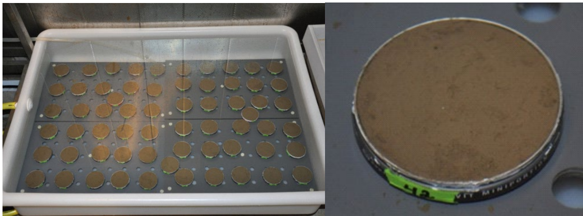
Figure 6. Experimental set-up at the Sven Lovén Center for marine sciences, with conditions similar to those in situ. The panel to the right shows a sediment plug (actual size).
