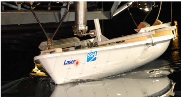
Figure 2. Photo by SSPA, showing the Laser dinghy during a run
