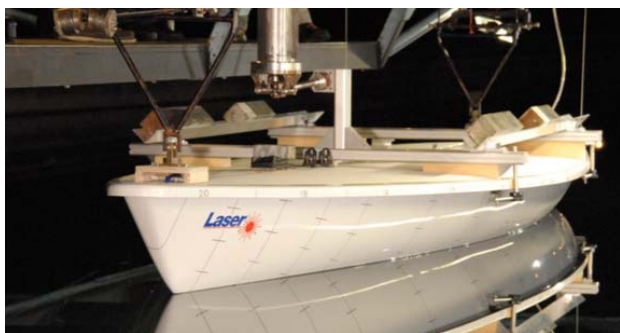
Figure 1. Photo by SSPA, showing the test-rig towing attachment and weights
