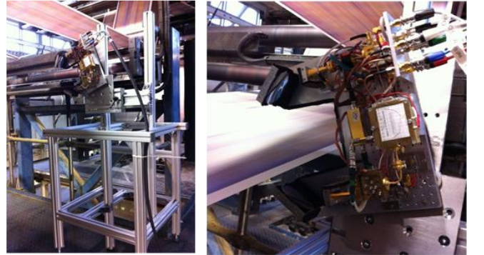
Fig. 10 Sensor location in the offset process. The beam is focused on the white strip at the edge of the paper.
