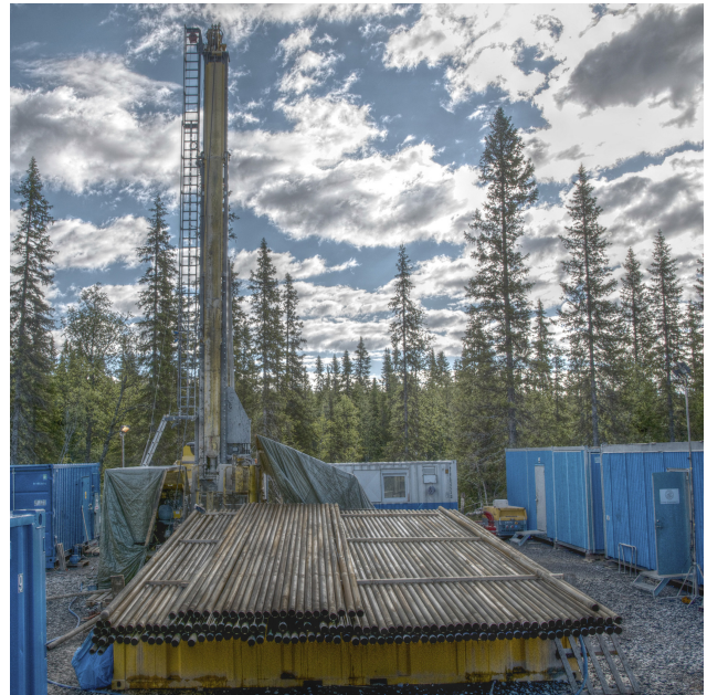
Figure 7. The Swedish national research infrastructure for scientific drilling, "Riksrigger". An Atlas Copco CT20C crawler mounted drill rig with a manual pipe handling system mounted on top of the mud tanks, with ca. 1400 m of HRQ drill pipe in this photograph.
