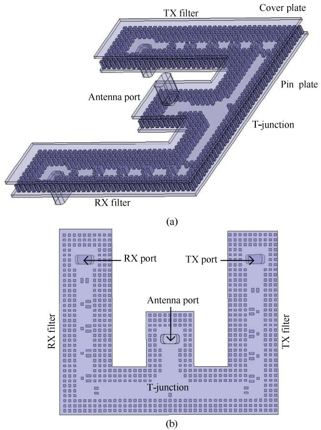
Fig. 1. Proposed 60GHz groove gap waveguide diplexer. (a) 3D view and (b) top view.
