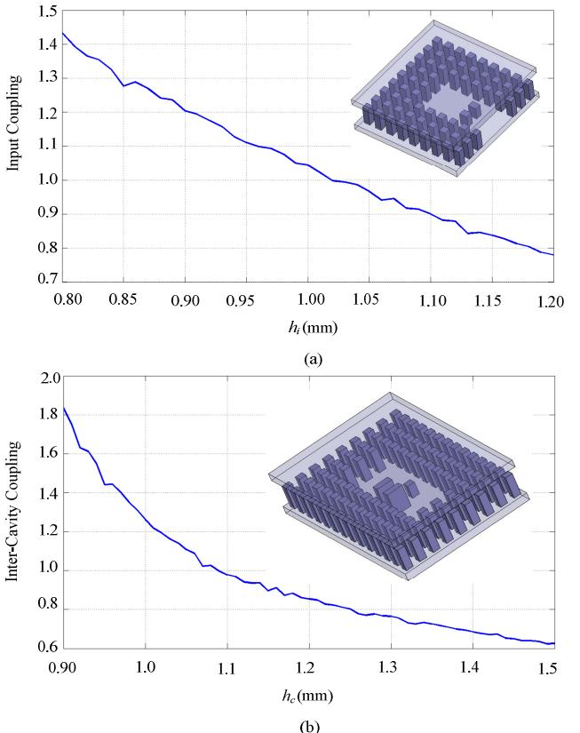
Fig. 4. (a) Input coupling coefficient,  $M_{Sl}$  (or  $M_{LS}$ ), versus height of ridge  $h_i$  and (b) inter-cavity coupling versus height of coupling pin  $h_c$ .
