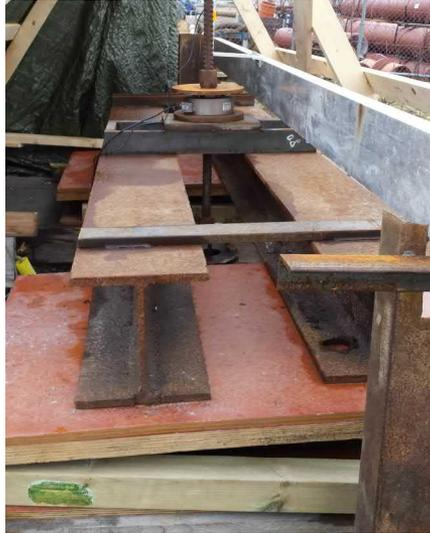
Figure 6.2: *Picture illustrating the tilting of the load frame to the left with reference to the timber mat.*
