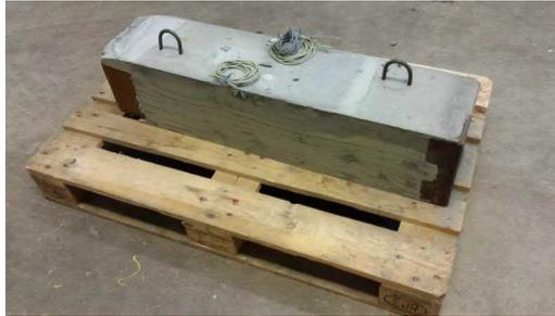
Figure A.7: *Model pile used to calibrate the strain gauges (1 m long).*
