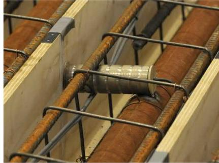
Figure 5.12: Pore water pressure transducer mount design at pile shaft.
