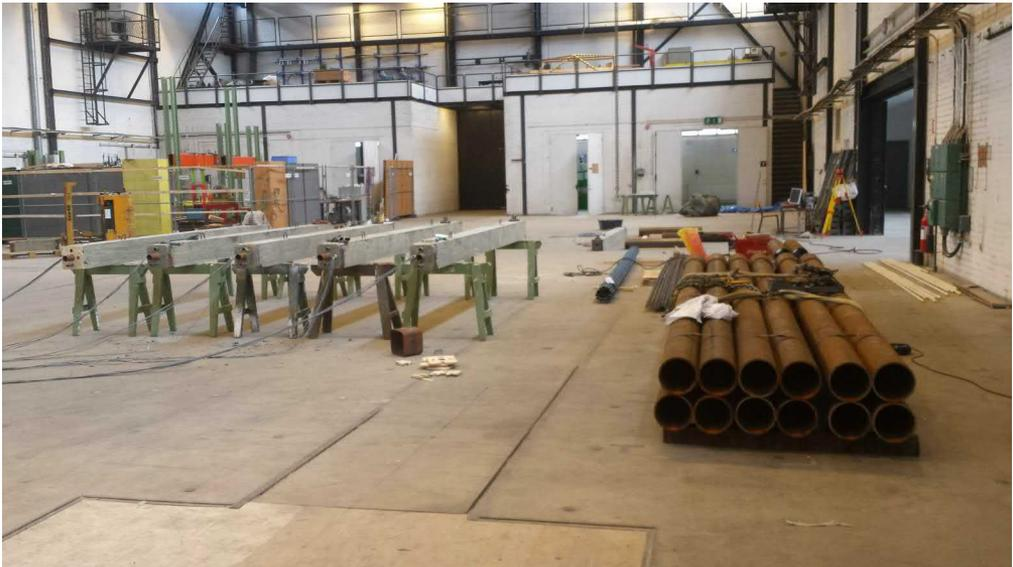
Figure A.9: *Concrete piles, steel extension piles, tell-tales and tension loading rod.*
