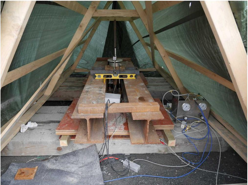
Figure A.11: *Load frame and manual pressure regulation panel.*
