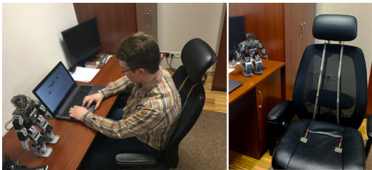
Fig. 4. The implementation of chair sensor during a second study - a Bioloid robot during the study on the left-hand side. Prototype sensors on the chair on the right-hand side.
