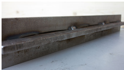
Fig. 3 Tack welded sample showing the cut arches and tack welds
