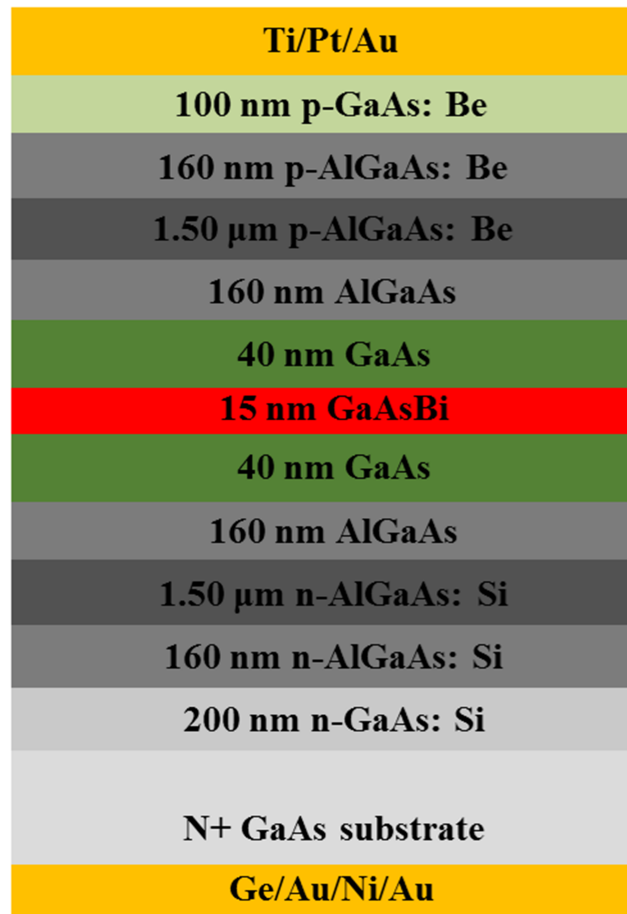
FIG. 1. Structure of GaAsBi QW LD.
