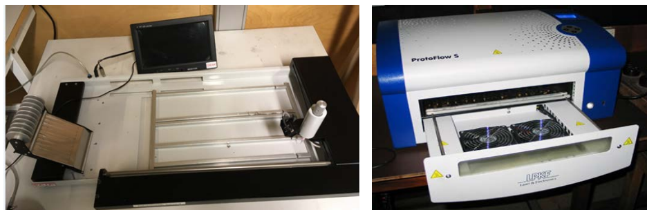
Figure 4. (a) Pick and Place Machine, (b) Reflow Oven.
