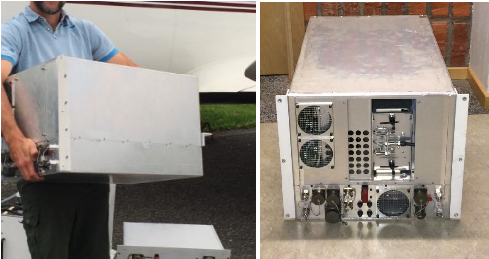
Figure 4. A custom designed FSC sniffer module. This box fits into a 19" rack, weighs 47 kg and utilizes 15 A at 28 V-DC. The system includes all instruments needed to monitor the FSC of ships from the air, i.e. a logging computer, AIS receiver, GPS receiver, power converter, calibration gases, \text{SO}_2 sensor, \text{CO}_2 sensor and pressure regulators. It is also the central system in the measurement system in the Navajo Piper aircraft.
