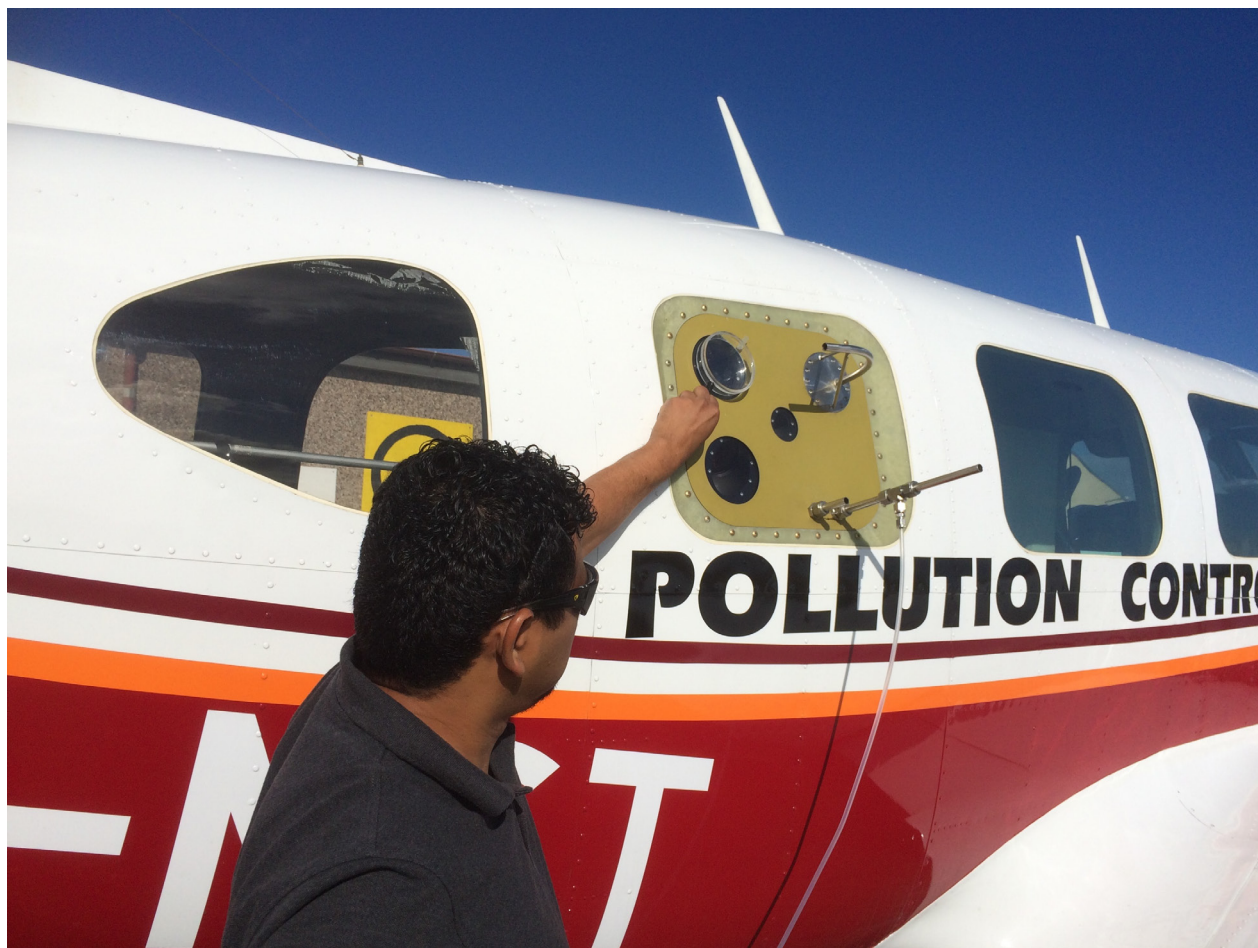
Figure 8. Quality control of the sniffer and optical sensors on the Navajo Piper aircraft from Aircraft Aps. The yellow plate includes two windows for optical sensors, a window for a video camera, two inlets for gases and particles, respectively, and one exhaust pipe. The optical system is checked by holding gas cells filled with known concentrations of \text{SO}_2 and \text{NO}_2 in front of the telescopes. The sniffer system is calibrated by flushing premixed calibration gas in front of the gas inlet using Teflon tubing.
