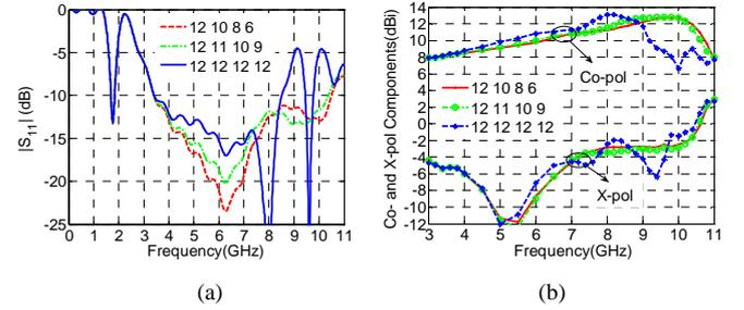
Fig. 5. (a)  $S_{11}$  and (b) co-polar directivity and cross-polar directivity vs. different y-axis width directors. The marking of 12 10 8 6 means the width of the 1<sup>st</sup> (closest to the driver dipole), 2<sup>nd</sup>, 3<sup>rd</sup> and 4<sup>th</sup> director, respectively.
