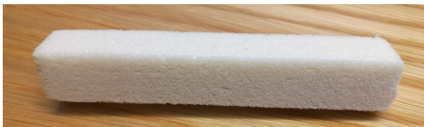
Figure 3.1: Rectangular sample with dimension 100 x 20 x 18 mm used for accelerated thermal aging of PUR.
