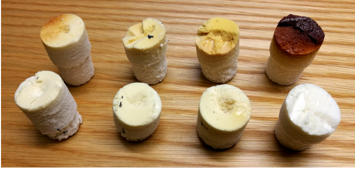
Figure 4.14: Samples from DHPs aged in air (upper row) and in N_2 environment (lower row) at 150^\circ\text{C} . The samples correspond to 840, 1680, 2520 and 3360 h of accelerated ageing time (from left to right).
