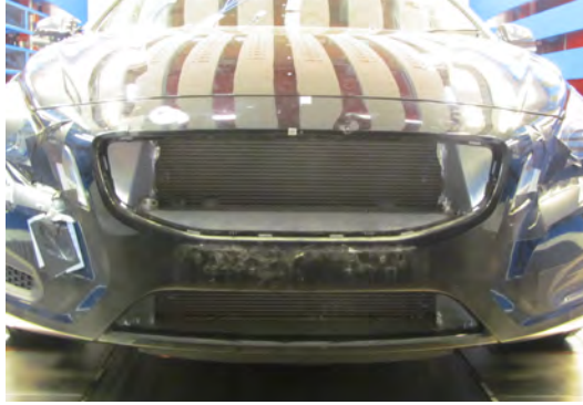
Figure 3.6: Reference configuration showing the aluminium ducts
