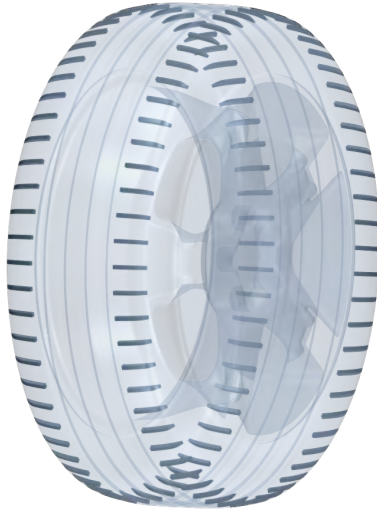
Figure 2.5: The MRF region, coloured in grey, in the improved MRFg method.
