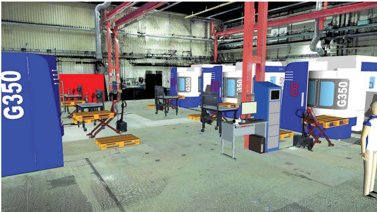
Figure 6-3: Realistic 3D layout of the planned production system.
