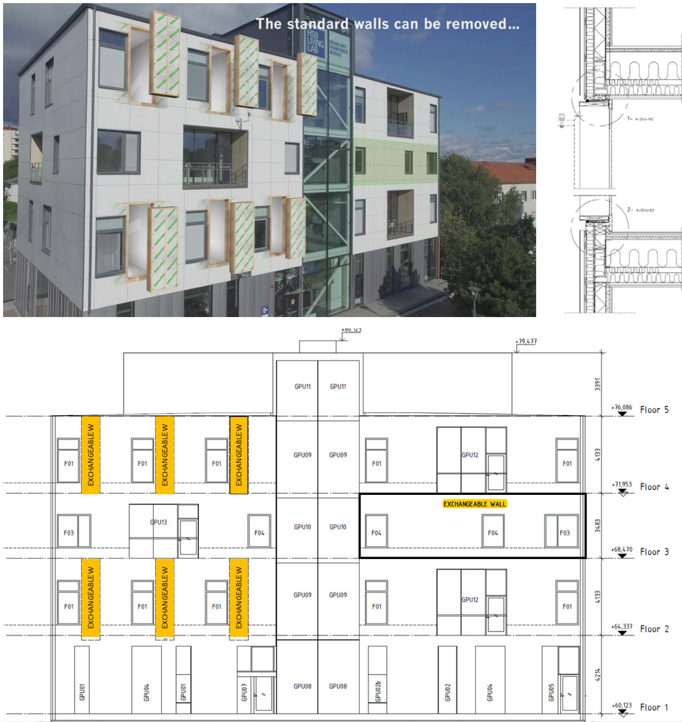
Figure 3. To the left: the position of six exchangeable walls of size 1.2x3.8 m on the west side of the building, on the second and the fourth floor. The light-green area on the third floor indicates another fully exchangeable exterior wall of size 12x3 m. Animation by Eyebright. To the right: a photo showing the exchangeable and the reference wall during the construction in a factory.
