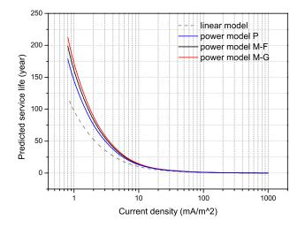
Figure 5.22: Predicted service life using the power model in comparison with the linear model.
