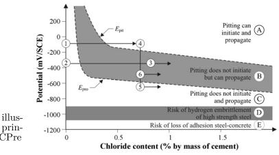
Figure 2.4: Schematic illustration of the working principles of ICCP and ICCPre (Bertolini et al. 2009).
