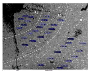
Figure 5.8: Back-scattered SEM spot analysis of the ring pattern formed around the anode.
