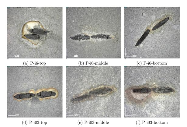
Figure 5.4: Typical leaching patterns of specimen's cross section for paste groups. The current density is listed in Table 3.5.
