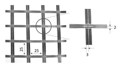
Figure 3.1: CFRP meshes as anode material. All values are in mm.
