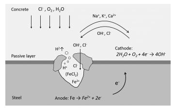
Figure 2.2: Schematic illustration of chloride induced pitting corrosion.
