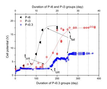
Figure 5.15: Potential monitoring of the paste groups. Dashed lines are fitted curves.
