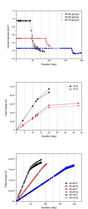
Figure 5.18: Current monitoring for the mortar groups. Dashed lines are fitted curves.
