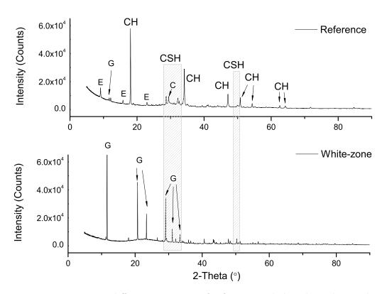
Figure 5.11: X-ray diffraction pattern of reference and the white-phase substance. Shadowed area indicates C-S-H phases. CH: Portlandite, Ca(OH)<sub>2</sub>; CSH: calcium silicate and C-S-H gel; E: Ettringite; G: Gypsum; C: Calcite, CaCO<sub>3</sub>.
