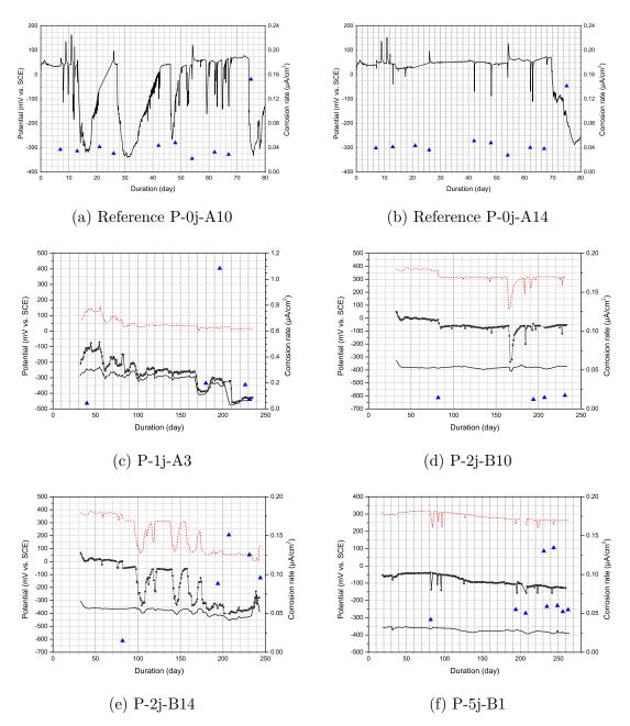
Figure 5.24: Examples of corrosion monitoring from each test group. Solid lines are the steel potentials (vs. SCE). Corrosion rates are measured by cathodic polarization ( $\blacktriangle$ ). The complete data is presented in Paper IV.
