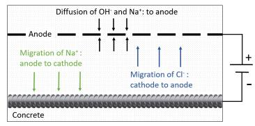
Figure 2.5: Schematic illustration of electrode reactions, migration and diffusion of ions (adopted from Bertolini et al. (2004))
