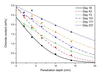
Figure 5.23: Chloride penetration profiles at different exposure times.
