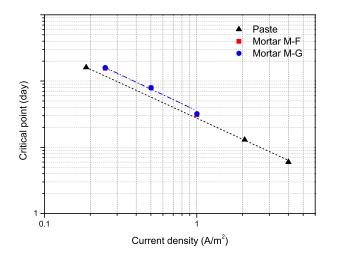
Figure 5.21: Critical turning point  $t_{crit}$  plotted against current density.
