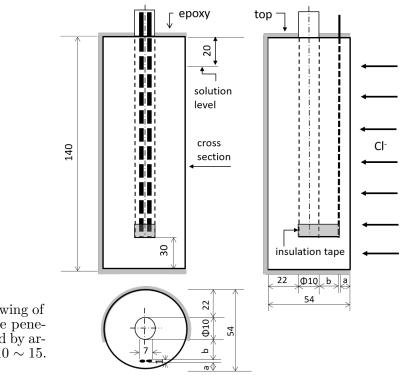
Figure 3.2: The 3-view drawing of a paste specimen. Chloride penetration direction is indicated by arrows.  $a = 7 \sim 10$  and  $b = 10 \sim 15$ . All values are in mm.
