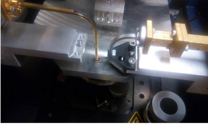
Figure 2.20: Measurement setup for the interconnect with the waveguide bend on the left and waveguide probe on the right
