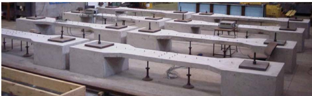
Figure 4.11 Geometry and dimensions of the restrained slab specimens and general view of the slabs during the testing period, from Nejadi and Gilbert [42].
