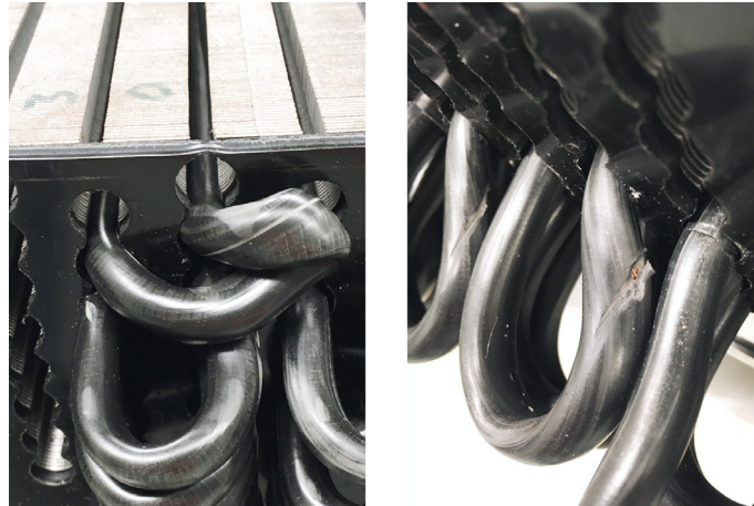
Fig. 14. Examples of failed robot-pulled end winding: a kinked end winding (left) and an end winding with a cut damage caused by the robot cable feeder tool during positioning against the next slot hole (right).
