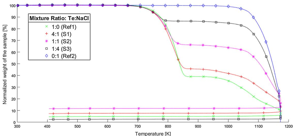
**Fig. 2** The thermogravimetric analysis results for the different Te:NaCl-ratios (weight basis) heated in inert conditions. The different lines represent the average of three replicates of 1:0 (Ref1, green crosses), 4:1 (S1, red pluses), 1:1 (S2, pink stars), 1:4 (S3, black
