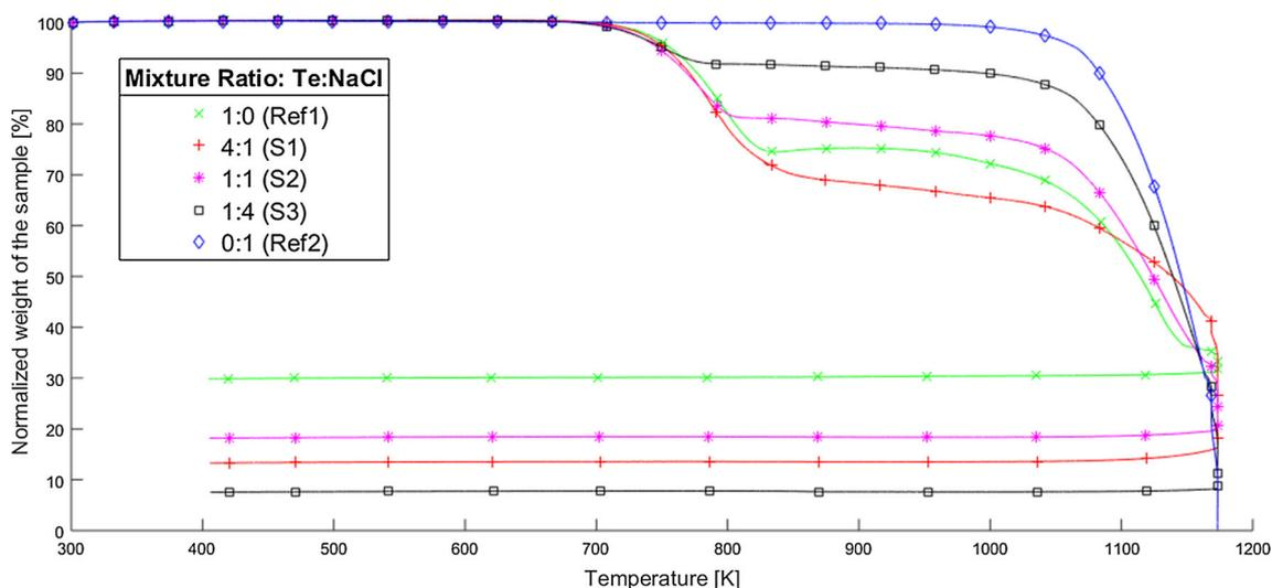
**Fig. 3** The thermogravimetric analysis results for the different Te:NaCl-ratios (weight basis) heated in oxidizing conditions. The different lines represent the average of three replicates 1:0 (Ref1, green crosses), 4:1 (S1, red pluses), 1:1 (S2, pink stars), 1:4 (S3, black
