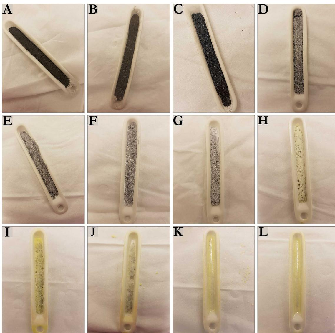
**Fig. 4** Crucibles containing the sample, as seen after the furnace experiment. The initial composition of the samples was 1:1 of tellurium and sodium chloride (2 g). In total eight, temperatures were
