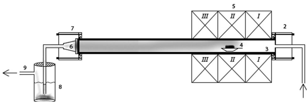
**Fig. 1** The experimental setup used: (1) gas flow inlet, (2) cylindrical formed inlet connector made from stainless steel, (3) ceramic tube of length 130 cm, (4) the mixture of compounds, (5) tubular furnace (6) filter holder, (7) cone formed outlet connector made from stainless steel, (8) cold trap used to prevent particles escaping, and (9) gas flow
