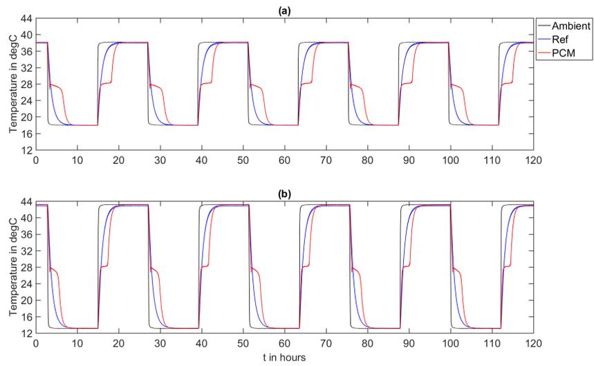
Figure Appendix A.2: T-History measurements of RT28HC for setup B1: (a): B1-I, (b): B1-II (all three sensor positions for reference and PCM are plotted with the same color, respectively)
