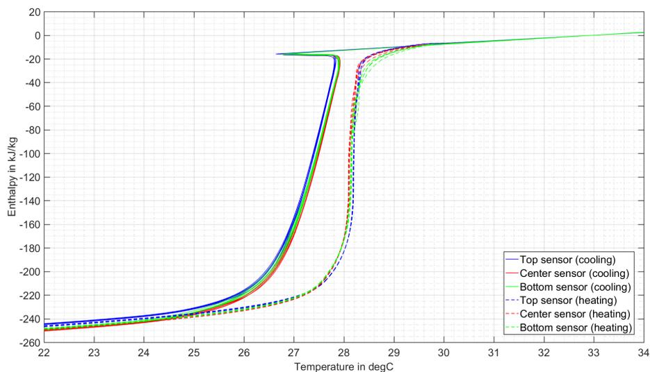
Figure Appendix B.4:  $h$  versus  $T$  curve for setup B1-II using  $dT = 0.001^\circ\text{C}$  (all five cycles are plotted with the same color depending on the sensor position, normalization of  $h$  values at  $33^\circ\text{C}$ )
