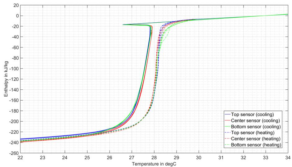
Figure Appendix B.1:  $h$  versus  $T$  curve for setup A-I using  $dT = 0.001^\circ\text{C}$  (all five cycles are plotted with the same color depending on the sensor position, normalization of  $h$  values at  $33^\circ\text{C}$ )
