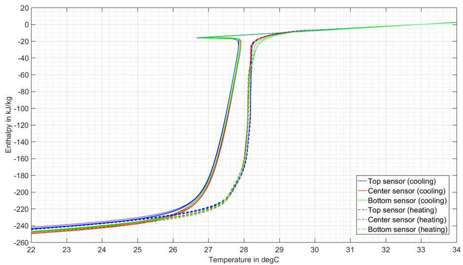
Figure Appendix B.3:  $h$  versus  $T$  curve for setup B1-I using  $dT = 0.001^\circ\text{C}$  (all five cycles are plotted with the same color depending on the sensor position, normalization of  $h$  values at  $33^\circ\text{C}$ )
