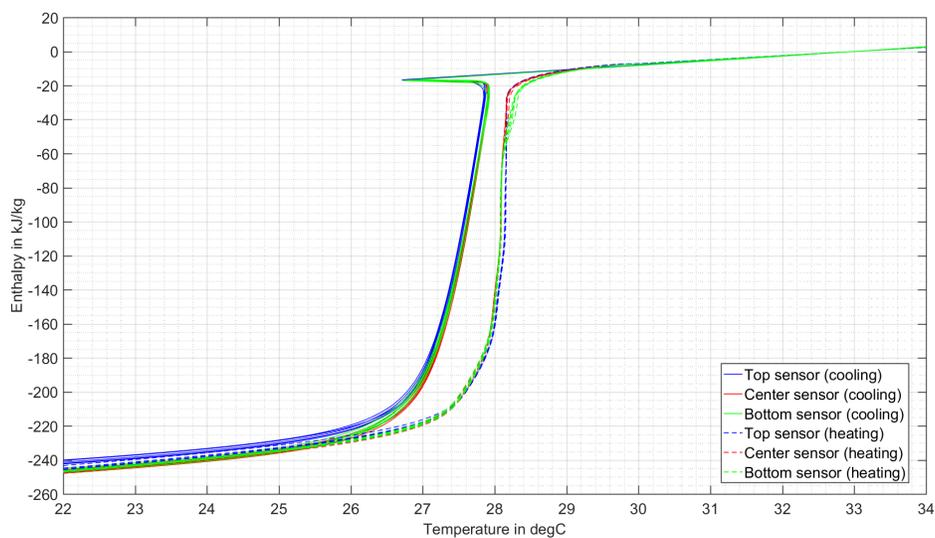
Figure Appendix B.5:  $h$  versus  $T$  curve for setup B2-I using  $dT = 0.001^\circ\text{C}$  (all five cycles are plotted with the same color depending on the sensor position, normalization of  $h$  values at  $33^\circ\text{C}$ )
