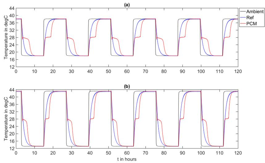
Figure Appendix A.3: T-History measurements of RT28HC for setup B2: (a): B2-I, (b): B2-II (all three sensor positions for reference and PCM are plotted with the same color, respectively)
