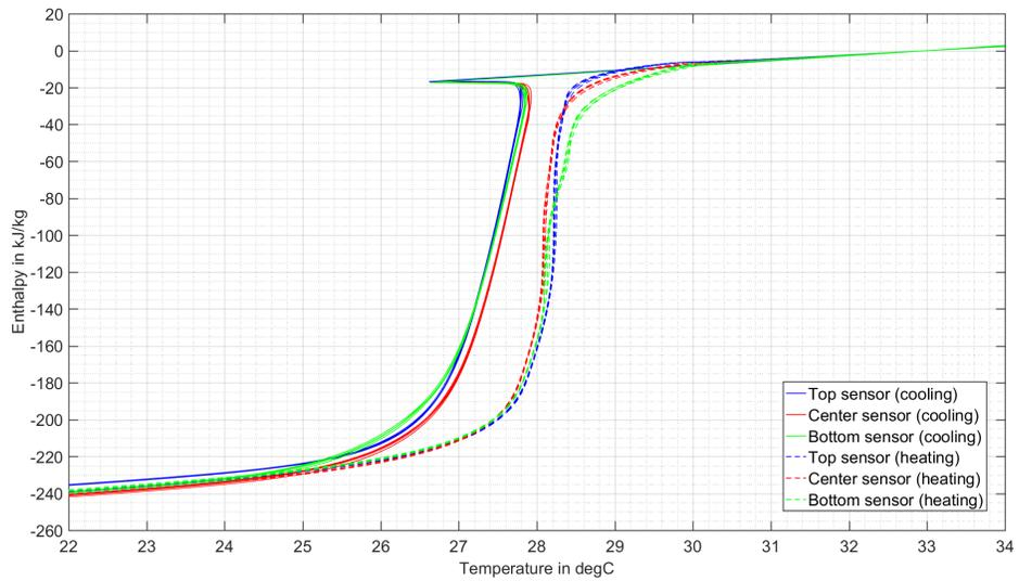
Figure Appendix B.2:  $h$  versus  $T$  curve for setup A-II using  $dT = 0.001^\circ\text{C}$  (all five cycles are plotted with the same color depending on the sensor position, normalization of  $h$  values at  $33^\circ\text{C}$ )
