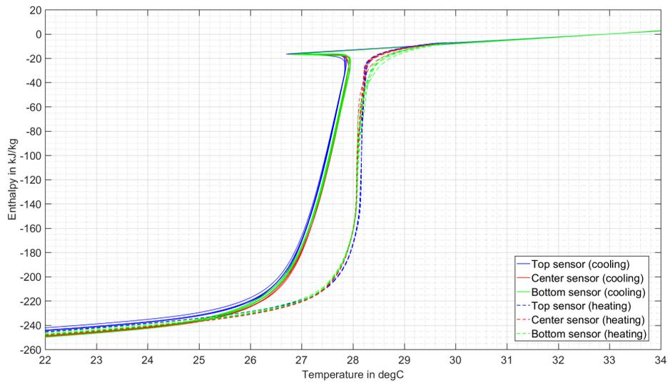
Figure Appendix B.6:  $h$  versus  $T$  curve for setup B2-II using  $dT = 0.001^\circ\text{C}$  (all five cycles are plotted with the same color depending on the sensor position, normalization of  $h$  values at  $33^\circ\text{C}$ )
