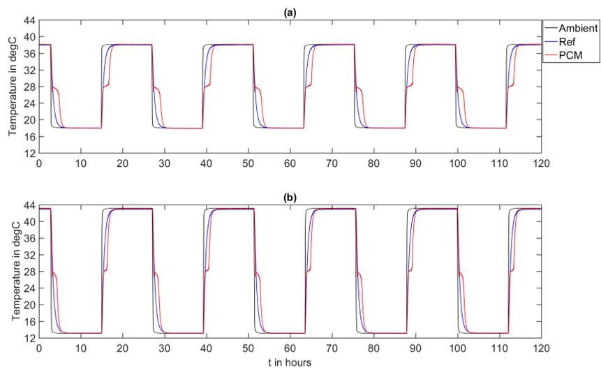
Figure Appendix A.1: T-History measurements of RT28HC for setup A: (a): A-I, (b): A-II (all three sensor positions for reference and PCM are plotted with the same color, respectively)
