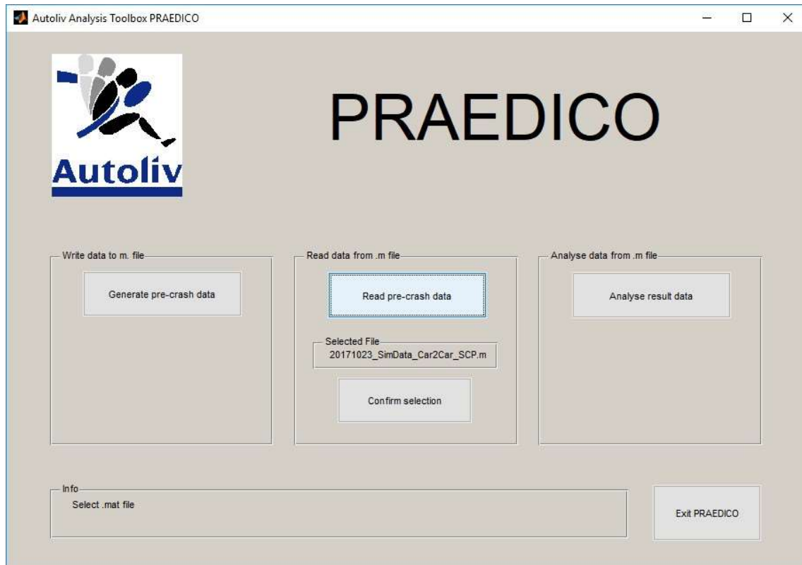
Figure B.1: PRAEDICO main GUI of PRAEDICO. In this GUI three different actions can be selected: A) Select data source and convert data to a Matlab file. B) Select Matlab data file for pre-crash simulation. C) Select Matlab simulation result file for analysis.
