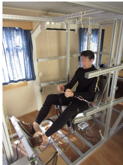
Fig. 5. MVC test rig with volunteer.
