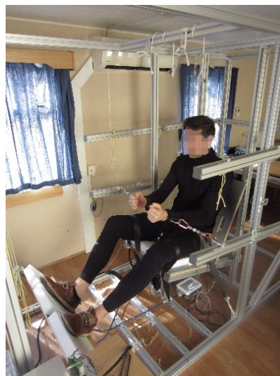
Fig. 5. MVC test rig with volunteer.
