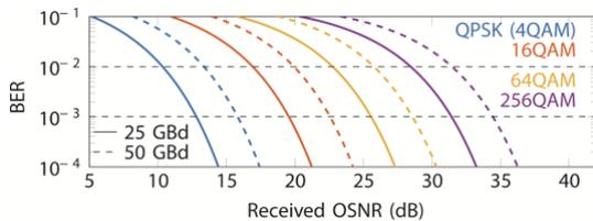
**Fig. 2:** Bit error ratio as function of received optical signal to noise ratio (0.1 nm bandwidth) for different modulation formats and symbol rates. Simulations assume Gray coding and additive white Gaussian noise.
