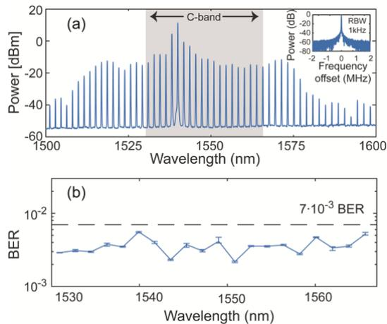
**Fig. 3:** (a) Optical spectrum of a 230 GHz microresonator comb. Inset denotes the line spacing stability measured by electro-optic downconversion. (b) Achieved BER upon propagation in 80 km single-mode fiber when encoding 20 GBd PM-64QAM data onto individual the comb lines within the C band<sup>9</sup>.
