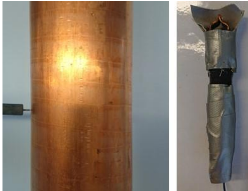
Figure 4-4. Left: Constantan needle measuring the copper tube wall temperature. Right: Beaker used to measure the bulk temperature. The reddish-brown parts are made of copper and the grey part in the front is a rubber cup capable of holding 10 ml, enough to fully submerge the copper plate with liquid. The constantan needle is inserted through a bottom hole in the cylinder handle until it touches the copper plate, closing the circuit of the thermocouple.
