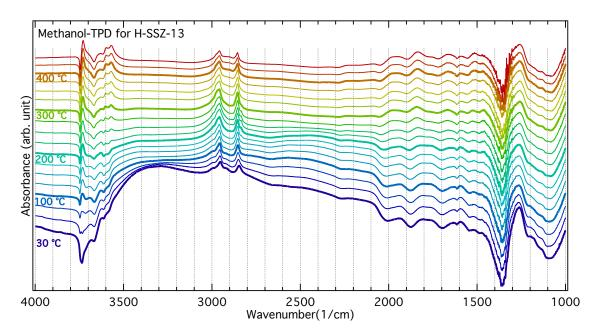
Figure S11: Infrared spectra collected during temperature programmed desorption of methanol from the H-SSZ-13 sample ramping the temperature from 30 to 450 °C.
