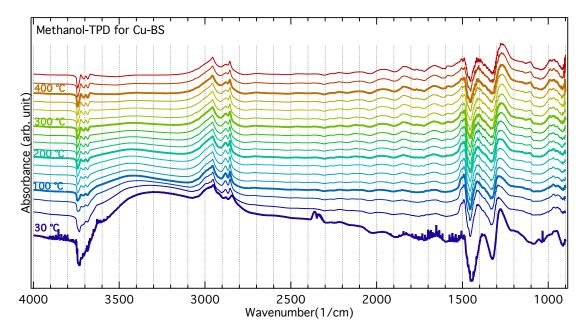
Figure S13: Infrared spectra collected during temperature programmed desorption of methanol from the Cu-BS sample ramping the temperature from 30 to 450 °C.
