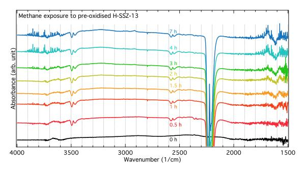
Figure S7: Infrared spectra for pre-oxidised H-SSZ-13 exposed to methane at 250 °C during 0 to 7 h. The spectrum at 0 h was taken in presence of 500 ppm of  $N_2O$  whereas the remaining spectra were recorded in Ar.
