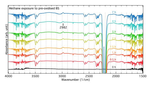
Figure S5: Infrared spectra for pre-oxidised BS exposed to methane at 250 °C during 0 to 7 h. The spectrum at 0 h was taken in presence of 500 ppm of  $N_2O$  whereas the remaining spectra were recorded in Ar.
