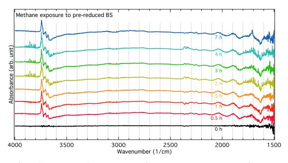
Figure S6: Infrared spectra for pre-reduced BS exposed to methane at 250  $^{\circ}$ C during 0 to 7 h. All spectra were recorded in Ar.
