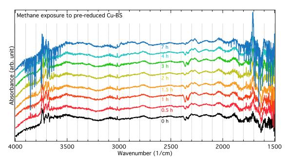
Figure S10: Infrared spectra for pre-reduced Cu-BS exposed to methane at 250 °C during 0 to 7 h. All spectra were recorded in Ar.
