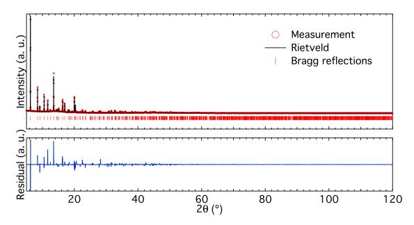
Figure S2: High-resolution X-ray diffractogram (upper panel) and Rietveld refinement (lower panel) for the BS sample.
