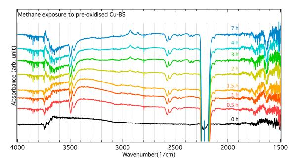
Figure S9: Infrared spectra for pre-oxidised Cu-BS exposed to methane at 250 °C during 0 to 7 h. The spectrum at 0 h was taken in presence of 500 ppm of  $N_2O$  whereas the remaining spectra were recorded in Ar.
