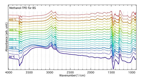
Figure S12: Infrared spectra collected during temperature programmed desorption of methanol from the BS sample ramping the temperature from 30 to 450  $^{\circ}$ C.
