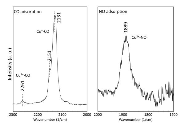
Figure S4: Infrared spectra recorded after CO adsorption (left) and NO adsorption (right) on the Cu-BS sample.
