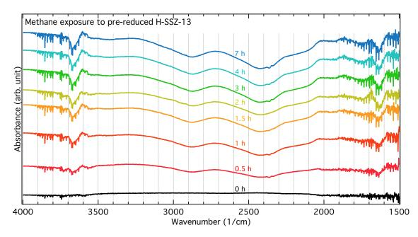
Figure S8: Infrared spectra for pre-reduced H-SSZ-13 exposed to methane at 250  $^{\circ}$ C during 0 to 7 h. All spectra were recorded in Ar.
