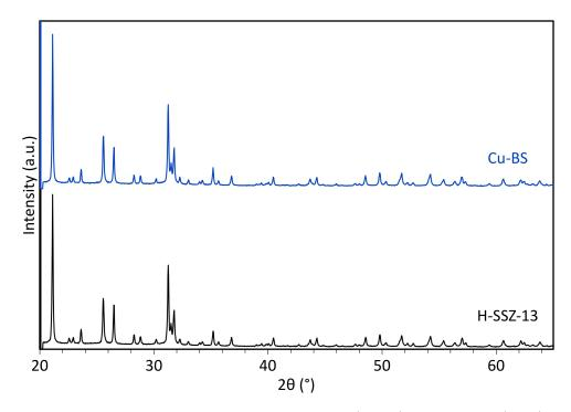
Figure S1: X-ray diffractograms for the H-SSZ-13 (black) and Cu-BS (blue) samples.
