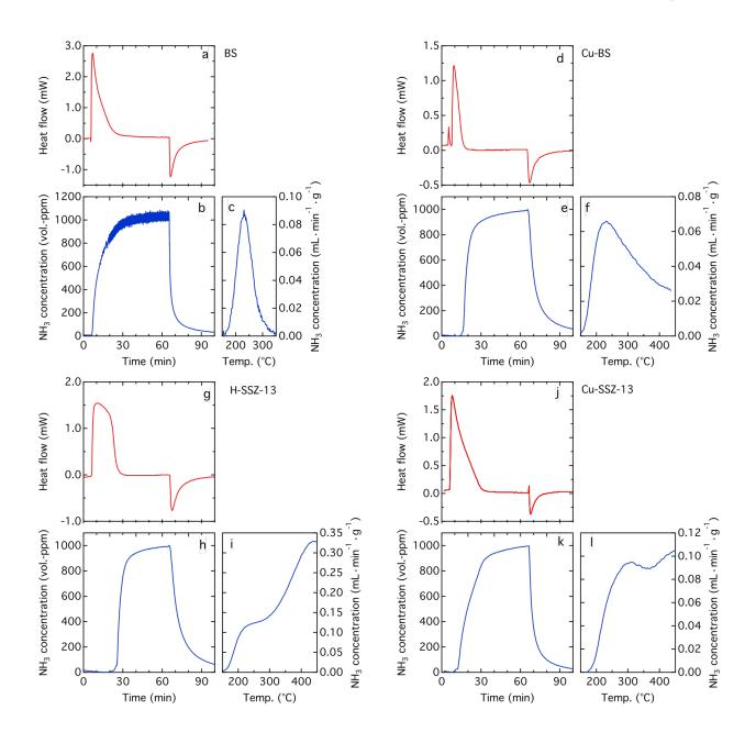
Figure S3: Thermogram (a, d, g, j) and ammonia mass spectrometer signal during NH<sub>3</sub> adsorption (b, e, h, k), and NH<sub>3</sub> desorption profile during linear heating (c, f, i, l) of the BS, Cu-BS, H-SSZ-13 and Cu-SSZ-13 sample.
