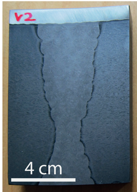
Figure 2.2: Cross-section of a pressurizer weld from Ringhals. The inside (top part in photo) is clad with stainless steel to enhance corrosion resistance.
