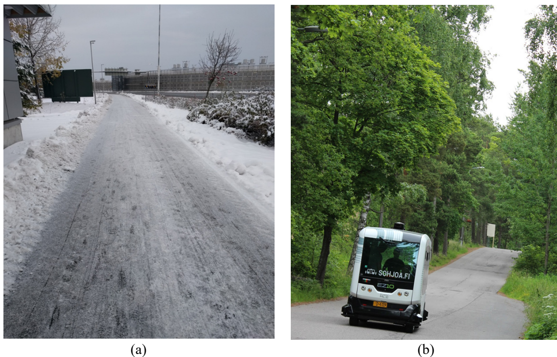
Figure 14. (a) Wintry weather stopped the operation in Helsinki pilot. The LiDARs of the robot bus see snow banks as obstacles. (b) An example of an area where the EZ10 robot bus localization does not work, as the trees are blocking the satellite connection and there are no fixed structures for the LiDARs.
