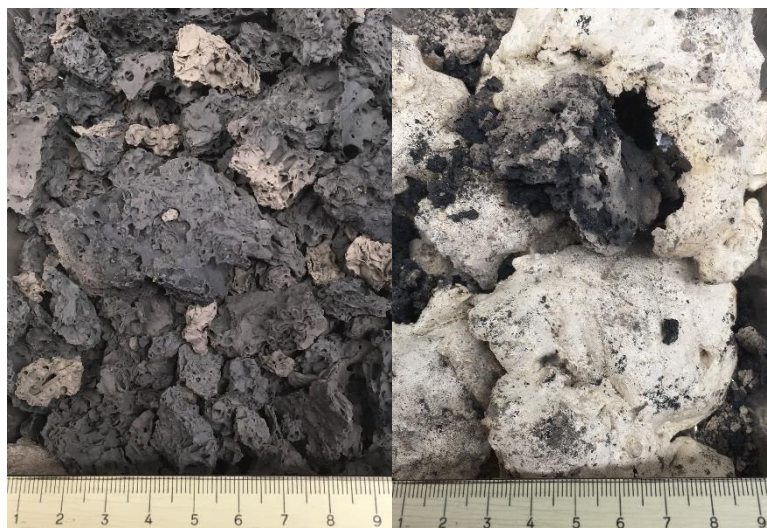
Figure 10 : a) Paint A and b) Paint B after microwave pyrolysis.
