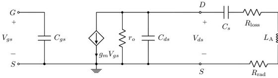
**Figure 6.** Small-signal equivalent circuit for the AiA.
