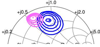
**Figure 2.** ADS simulated load-pull for maximum PAE for the HEMT at 30 GHz (magenta, left) and at 18 GHz (blue, right), contour interval: 5%. (Test conditions:  $V_{DS} = 28\text{ V}$ ,  $I_{DS} = 40\text{ mA}$ , bondwires excluded.)
