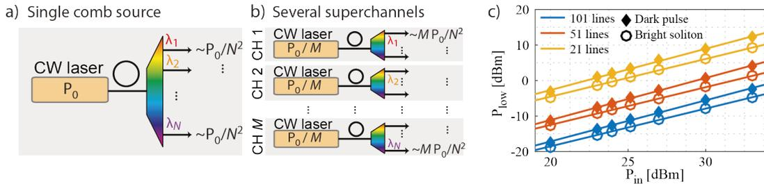
Fig. 1: The diagram in a) shows the single comb approach, providing  $N$  lines using a single comb and CW laser with pump power  $P_0$ . In b) the total optical power has been distributed between  $M$  lasers, each pumping a separate comb providing  $N/M$  lines. According to the nonlinear scaling law this solution yields  $M$  times more power per line than the single comb. The graph in c) shows the simulated performance of individual combs
