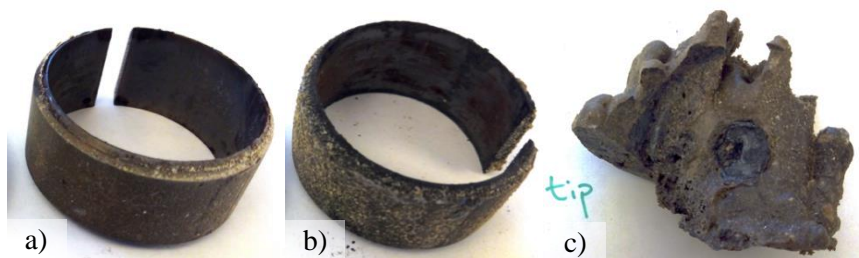
Figure 50: Photographs of three different amounts of deposits accumulated on Sanicro 28 for three different settings after 2-hour exposures. A) small amount, b) moderate amount, and c) large amount.
