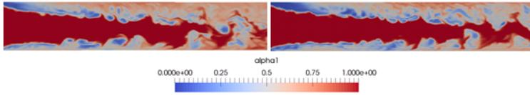
Figure 5.2: Instantaneous volume fraction from the stochastic field model on the left and single volume fraction solver on the right
