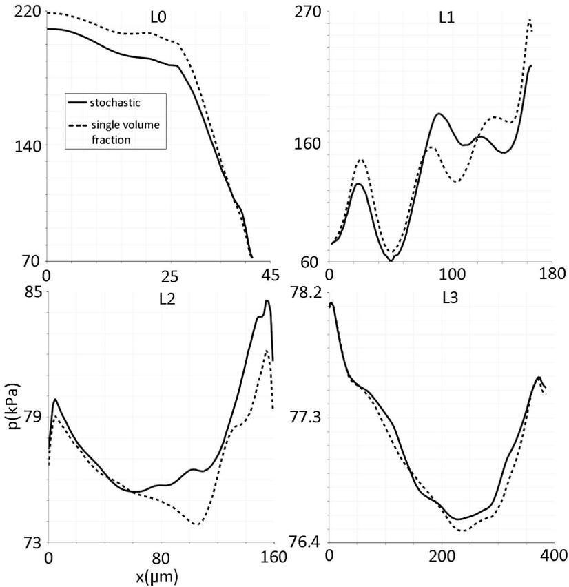
Figure 5.5: Time averaged pressure (kPa) along L0, L1, L2, and L3 as predicted by stochastic model (solid lines) and single volume fraction solver (dash lines)
