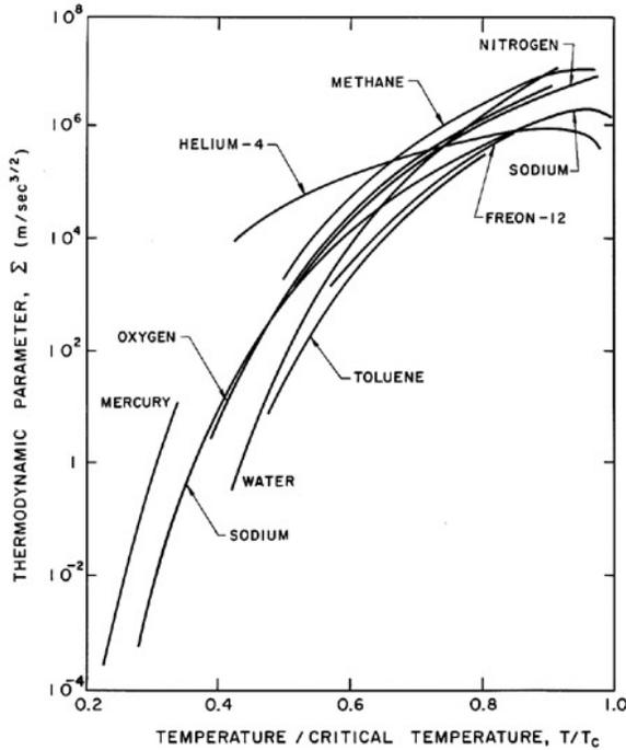
Figure 2.4: Values of the thermodynamic parameter,  $\Sigma$ , for various saturated liquids as a function of the reduced temperature,  $T/T_c$ .
