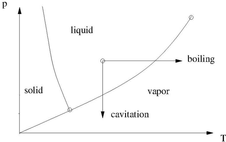
Figure 2.1: Cavitation and boiling demonstrated in p-T diagram
