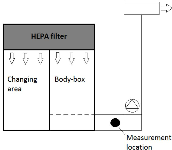
Figure 1. Principal arrangement of dispersal chamber (body-box).
