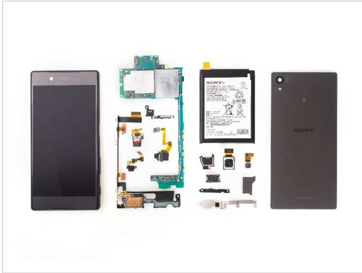
Figure 1: A disassembled Sony Xperia Z5. Source: iFixIt webpage
