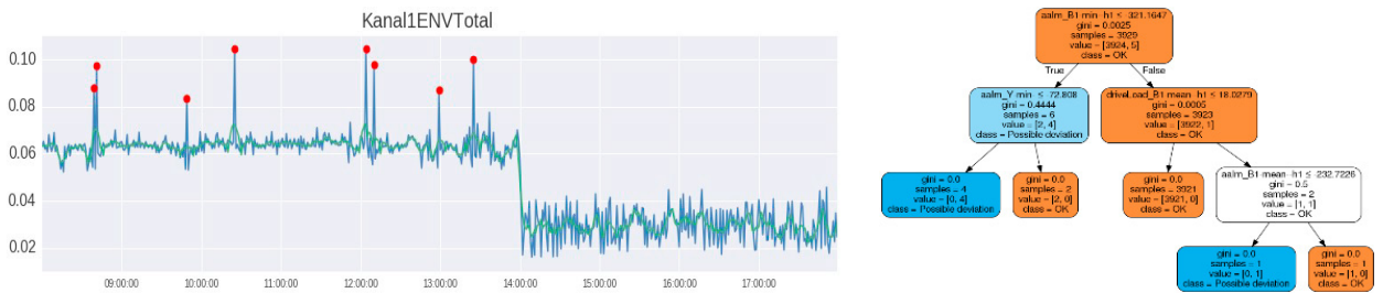
Figure 4: Left: Detected anomalies marked in red for one vibration sensor, Kanal1ENVTotal (data blue, smoothed data green). Right: Decision Tree for a sensor with five detected anomalies (deviations). Blue boxes show on value combination for deviations.
