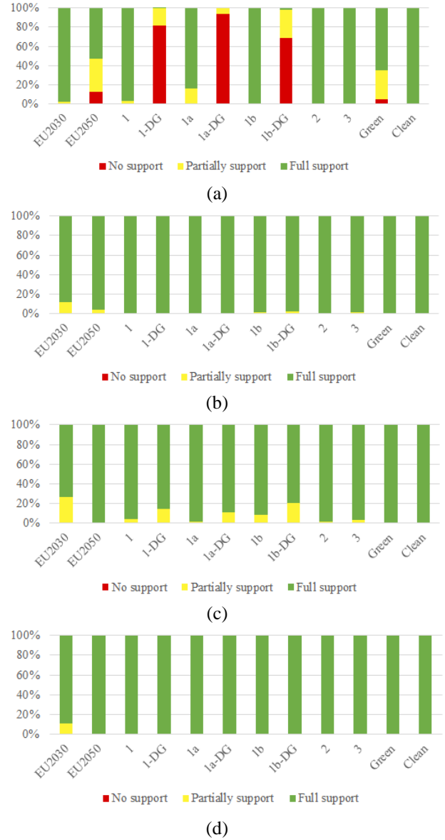
Figure 4. Wind power contribution on inertia support for the (a) UCTE, (b) Nordic, (c) UK and (d) Baltic synchronous grids.
