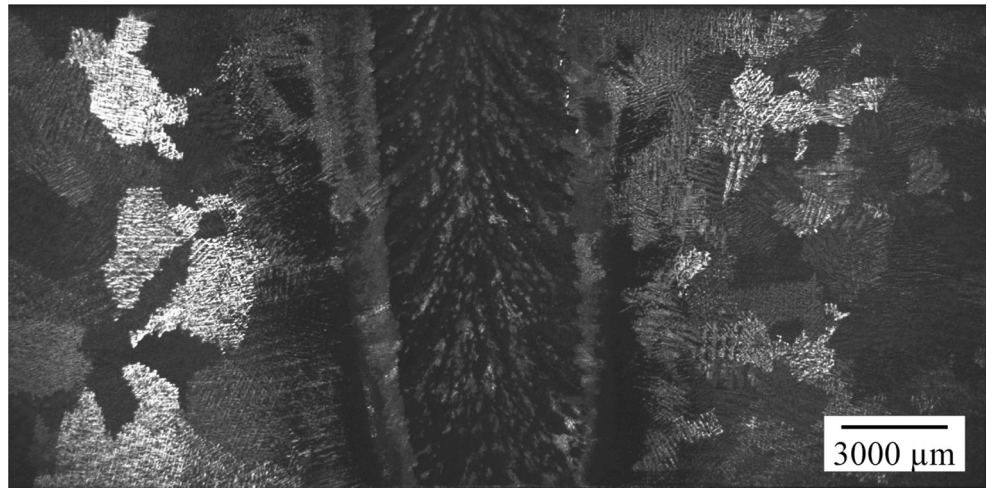
Fig. 8 Grain structure of an as-cast test plate
