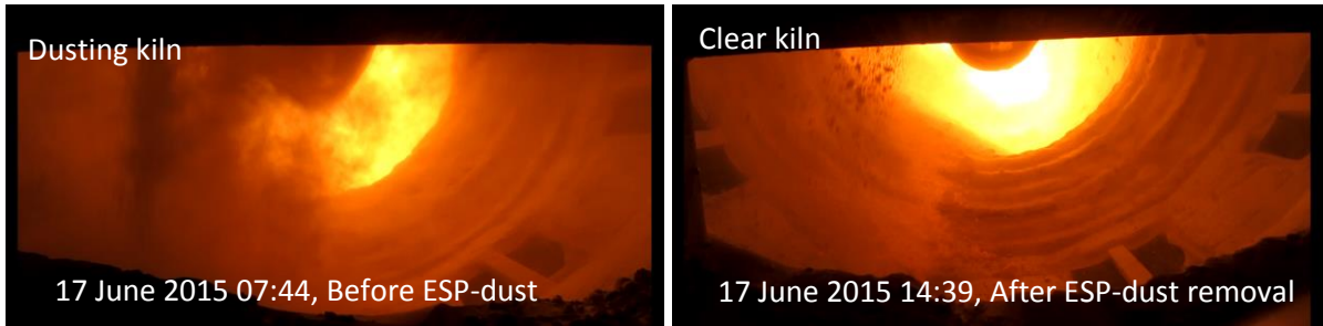
Figure 23: Before removal of ESP dust (left) and after removal of ESP dust (right) from 17 June 2015.
