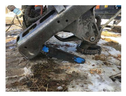
Figure 1. A typical position of the saw when changing the saw chain on a harvester head
